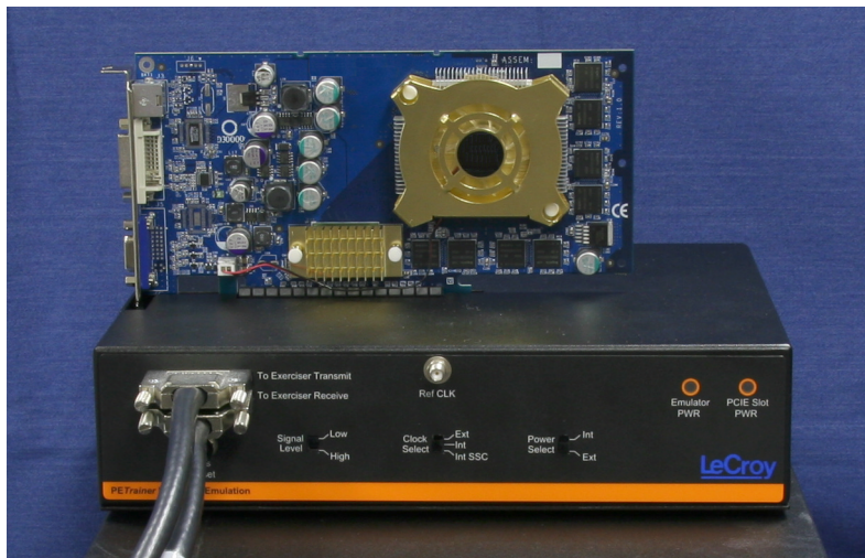
Host emulation test fixture with a PCI-E graphics card on top.
